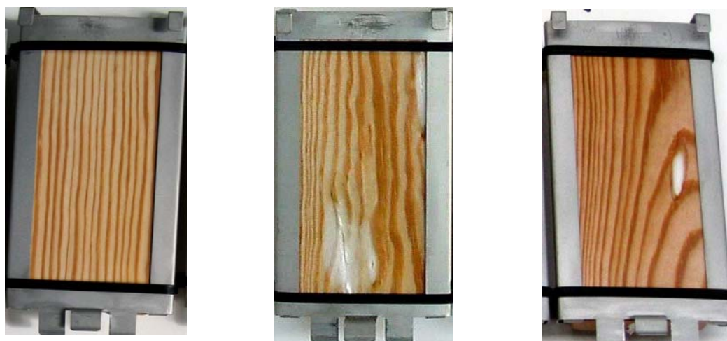
Figure 5. Artificial weathering (Xenon) of coated wood (pine) after 2000 hours, from left to right: polycarbonate(K), polyester (A) and acrylic latex (industry standard)
