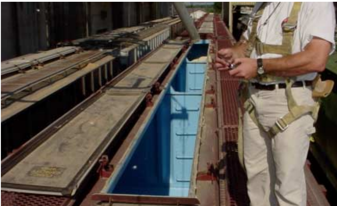
Figure 1. View of hopper car compartments during filling
