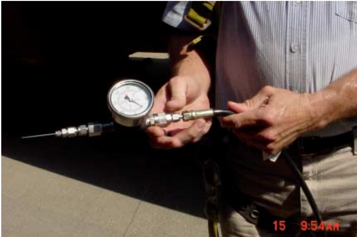
Figure 3. ECO 2 FUME® nozzle tip assembly
