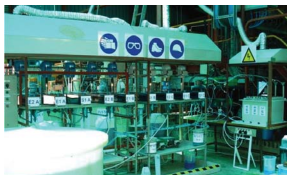
Figure 1 Pilot Plant Unit: Three side-by-side closed circuit SXEW operations.
